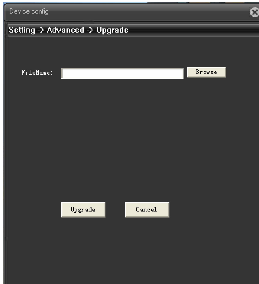
Pic: 4.41 system upgrade
