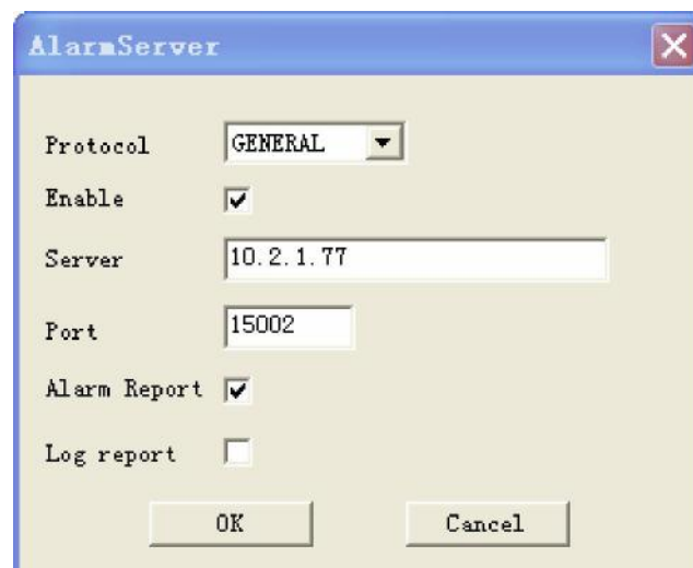
Pic: 4.25 Alarm center setting
