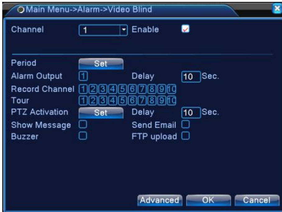
Video blind in full digital(NVR) mode
