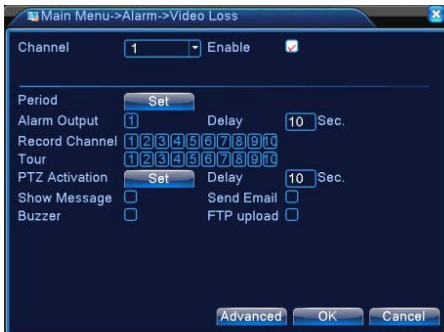
Video loss in Hybrid(HVR) mode
