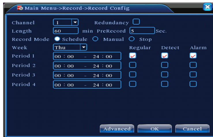
Picture 4.1 Record Configuration
