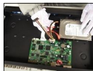
⑥ connect the power wire
