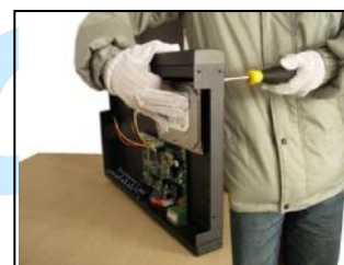
③ fix the screw of hard disk
