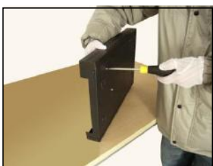
④ fix the screw of hard disk
